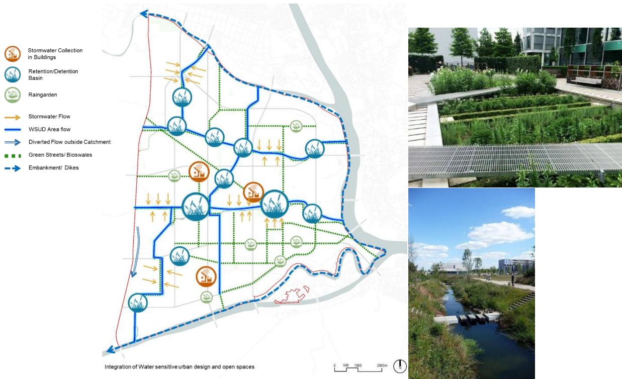
Figure 9: Water Sensitive Urban Design principles for storm water management across New Yangon City (by NYDC and AECOM).
